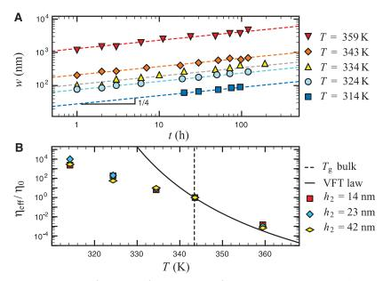
**Fig. 2.** Temporal evolution of the width of stepped films and temperature dependence of the **effective viscosity.** (**A**) The temporal evolution of the width w (see Fig. 1C), obtained by fitting the profile to a tanh[x/(w/2)] function, for talling has 1000 to 1000
