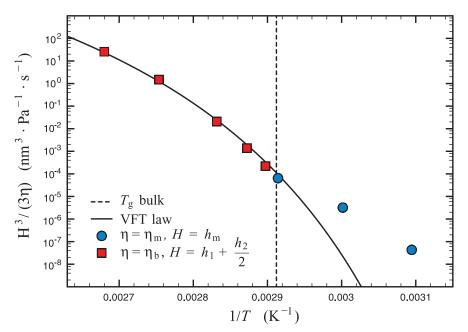
**Fig. 5. Temperature dependence of the mobility.** This figure is made of two subplots representing  $h_1 = h_2 = 90$ -nm samples. The mobility  $H^3/(3\eta)$  is determined by a fit to either the analytical GTFE solution (blue circles) or the numerical TFE solution (red squares), with  $\eta$  and H as defined in the legend.
