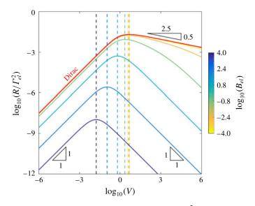
FIGURE 5. (Colour online) Normalized wave resistance  $R/\Gamma_{el}^2$ , as given by (3.5) and (4.4), as a function of the reduced speed V, for various elastic Bond numbers  $B_{el}$  as indicated. The Dirac limit  $(B_{el} \rightarrow 0)$  is indicated. The vertical dashed lines indicate the position of the maximal wave resistance (see (4.11)), for each value of  $B_{el}$ .
