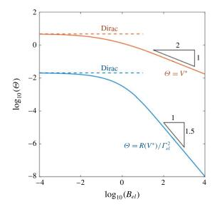
FIGURE 6. (Colour online) Computed values of the normalized maximal wave resistance  $R(V^*)/\Gamma_{el}^2$  (blue) and the corresponding speed  $V^*$  (red), as functions of the elastic Bond number  $B_{el}$ , according to (4.7) and (4.11). The dashed lines represent the Dirac limits given in (4.14) and (4.15).
