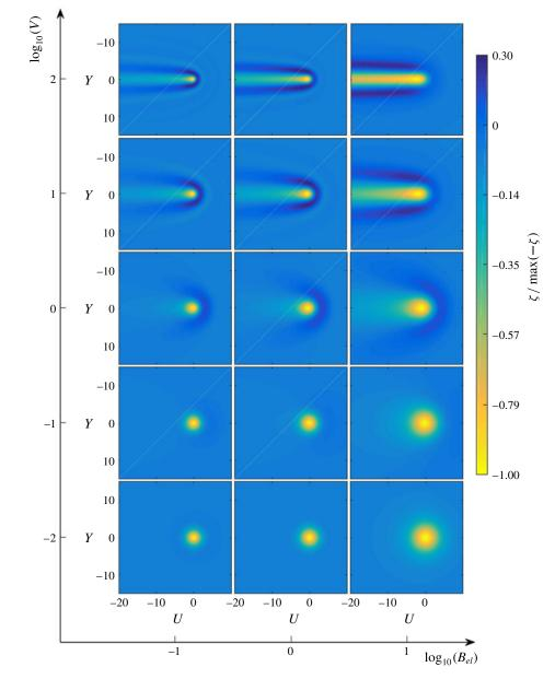
FIGURE 2. (Colour online) Top view of the normalized wake created by a Lorentzian pressure field, computed from (3.4) and (3.5), for different values of the elastic Bond number  $B_{el}$  and the reduced speed V as indicated (log is the natural logarithm). Since we use the comoving-frame variables, U = X - VT and Y, the pressure field is centred at U = 0 and the two-layer film travels at constant speed V from right to left in each panel.
