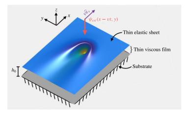
FIGURE 1. (Colour online) Schematic of the elastohydrodynamic wake. The top elastic film reacts to an external disturbance  $\psi_{ext}(x - vt, y)$  moving at constant speed  $v \ge 0$  along the x direction at time t.
