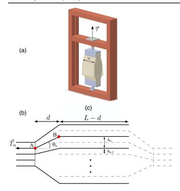
FIG. 1. The enigma of the two interleaved phone books: experimental setup and theoretical model. (a) Schematic of the experimental setup. (b) Schematic of the interleaved books introducing the local traction force  $T_n$  exerted by the operator on the nth paper sheet. The two vertical lines represent the clamps, while the other lines represent the central lines of each sheet.
