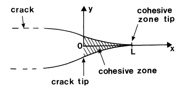
Figure 1. A schematic diagram of a cohesive zone ahead of a crack.
